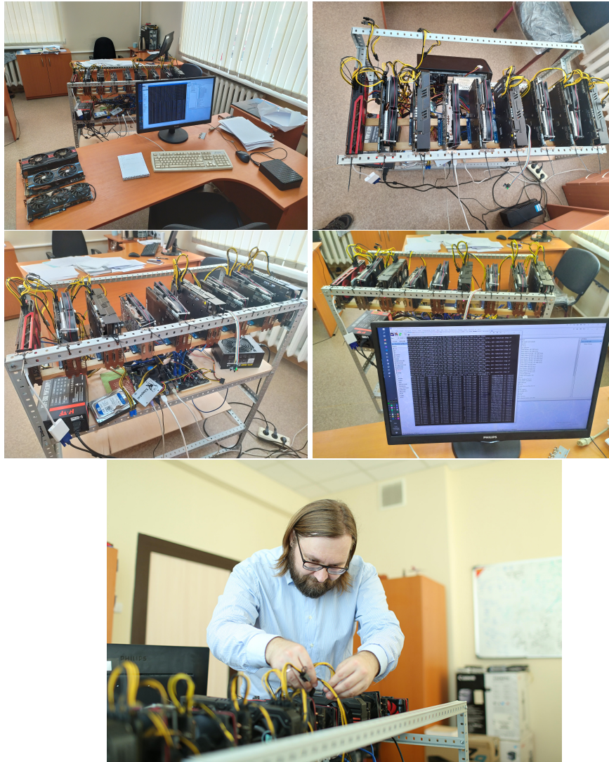
Figure 5.1: Workstation of ICRANet-Minsk center: 14 Tahiti chips, 14 TFLOPS in double precision
