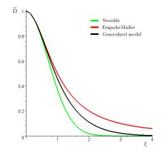
Figure 0.6: Dimensionless angular velocity versus dimensionless equatorial radius for the three models taken into exam.
