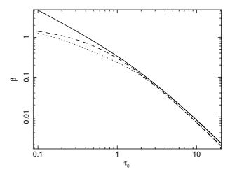
**Fig. 2.** Values of the  $\beta$ -parameter as a function of the optical depth  $\tau_0$ . The solid, dashed and dotted lines correspond to definition of  $\beta$  given in equations (15), (17) and (18), respectively.
