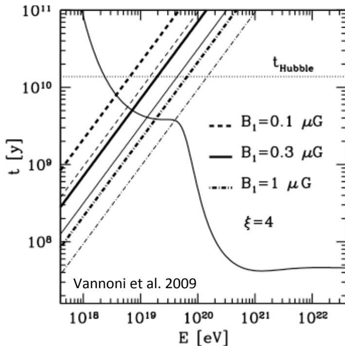
**Fig. 1.** Acceleration and energy loss time scales as a function of the proton energy. The acceleration time scales are obtained for the values of the upstream magnetic field  $B_1$  reported in figure and a downstream magnetic field  $B_2 = 4B_1$ . The thick lines correspond to a shock velocity of 2000 km/s, the thin lines to a velocity of 3000 km/s. As an horizontal dotted line we report the estimated age of the Universe, for comparison.
