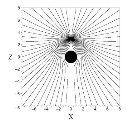
**Figure .3:** Lines of force of the effective electric field of the particle alone in the extreme case Q/M = 1 for the same choice of the distance parameter as in Fig. .1. No lines of force intersect the black hole horizon in this case, leading to the the "electric Meissner effect."
