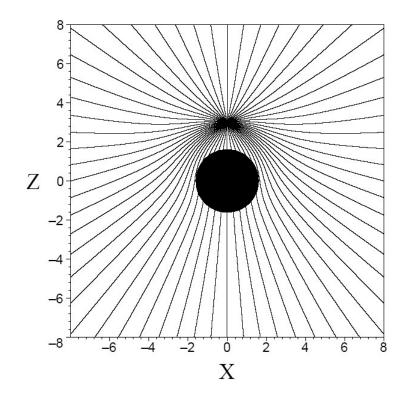
**Figure .2:** Lines of force of the effective electric field of the sole particle in the non-extreme case for the same choice of parameters as in Fig. .1. As explained in the text this "effective field" is obtained by subtracting the dominant contribution of the black hole own electric field to the total perturbed field, thus representing the net effect of the perturbation induced by the massive charged particle on the background field.
