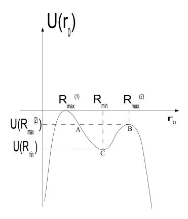
**Figure C.1.:** The membrane's motion can be described as the motion of a non-relativistic point particle in the potential  $U(r_0)$ .
